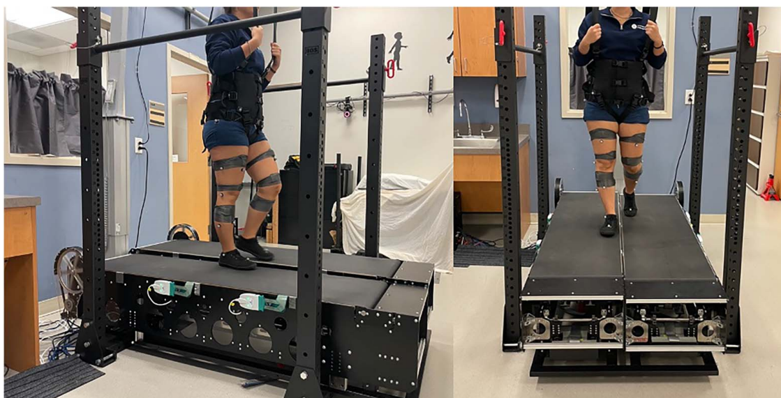
Fig. 1 The VST 2 with a subject walking on it while wearing a harness-based body weight support. The subject is equipped with 22 motion capture markers as well as 10 EMG electrodes tracking muscle activity. The left figure shows the right belt at a lower stiffness than the left, resulting in a vertical deflection. The right figure shows the opposite.
