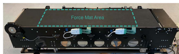
Fig. 5 One VST 2 platform with force mats installed
