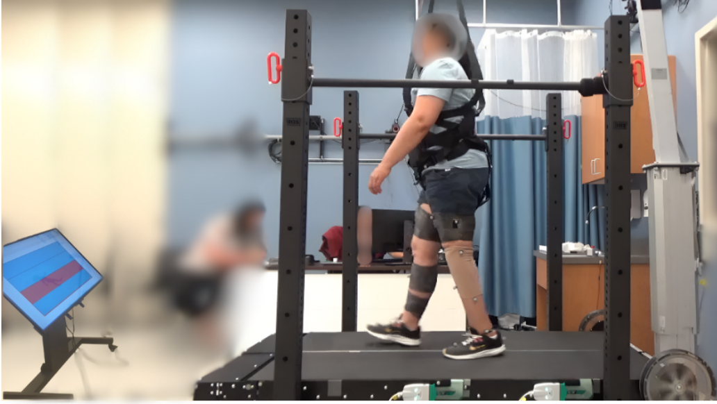
Figure 2: The experiment setup including a view of the VST 2 and the visual feedback monitor. Subject instrumentation is shown, including EMG electrodes and reflective motion capture markers. The image shows the TTA participant walking on the VST 2, preparing to transition to a low stiffness ( S_L ) surface with their left (prosthetic) leg.
