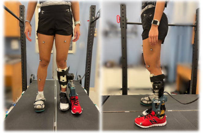
Fig. 2: Front and side view of a subject standing on the VST 2, while wearing the powered ankle-foot prosthesis Ruggedized Odyssey Ankle (ROA) attached to an ankle bypass adapter.
