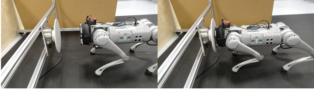
Fig. 8: Experimental sequence of the controlled pushing evaluation. Left: The quadruped robot in its initial pre-contact stance, positioned opposite the ATI force-torque sensor plate. Right: Active contact phase, illustrating the sensorized helmet engaging the force plate during dynamic fore-aft loading.
