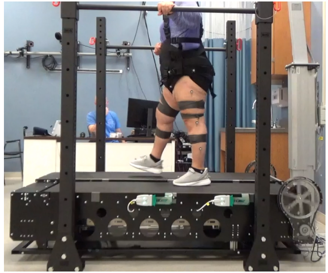
Fig. 1: The Variable Stiffness Treadmill (VST) 2 with the subject wearing motion capture markers, EMGs (under wraps), body-weight-support harness, and heart rate monitor (under harness). The left platform can be seen deflecting as the subject steps on it.
